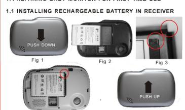
Fig 5 • Open battery compartment by pressing and pushing the battery cover down as show in Fig 1 • Insert rechargeable battery in the battery compartment as show in Fig 2. Align battery so the small plastic corner pieces above and below the metal pins in the battery compartment, align with the cut-out portions of the battery as show in Fig 3 and Fig 4. Close the battery compartment by aligning the cover with the battery compartment and pressing and pushing the cover up as
